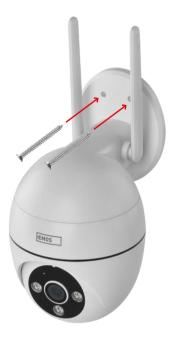
Use the supplied holder to place on a clean surface. Fasten with the supplied screws.
