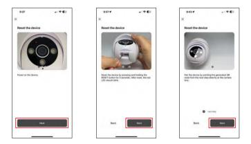
Turn on and reset the camera using the RESET button on the bottom of the camera and continue with the application. After a successful reset, the indicator should flash rapidly.
