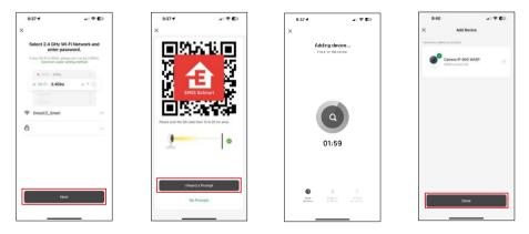
Enter the name and password of your Wi-Fi network. This information remains encrypted and is used to allow the camera to communicate with your mobile device remotely.
